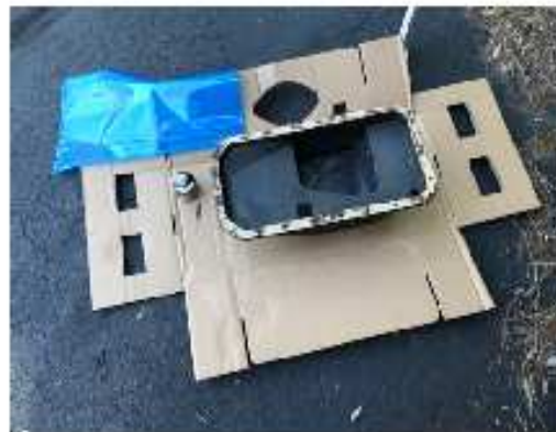
Cleaned up sump pan fitted with a new gasket.
