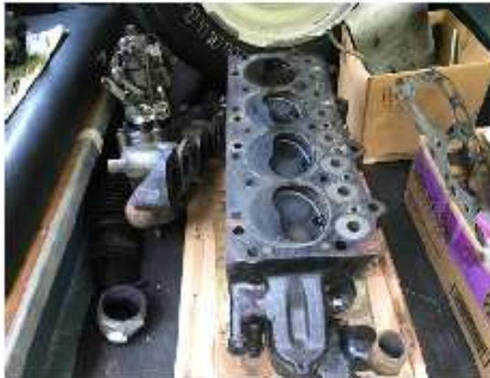
Parts storage in the back of the Rover: The head, showing exhaust and intake valves sitting next to the intake manifold with the Solex carburetor on top.
