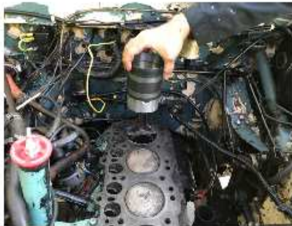
Jack with the piston ring compressor inserting the new piston and reused connecting rod assembly into cylinder #4.
