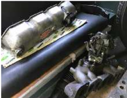
Parts storage in the back of the Rover: The head, showing exhaust and intake valves sitting next to the intake manifold with the Solex carburetor on top.
