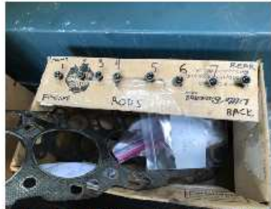
Cardboard box (with numbered slots) holding push rods in the correct order waiting for reinstallation; used head gasket as removed.
